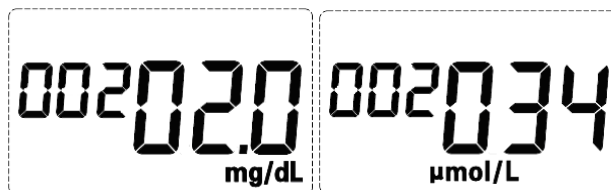
Figure 7- 3 Conversion of unit
